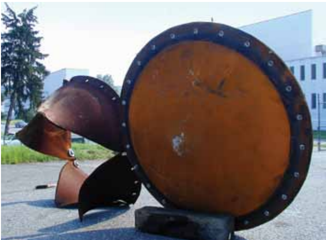
Blast tests carried out at US Navy's Naval Surface Warfare Center (NSWC) demonstrate how SPS absorbs more blast energy, reduces risk of premature rupture and limits fragment penetration. The conventional steel panel (left) is ruptured by the blast while the SPS panel (right) absorbs the energy and deforms without rupture.
