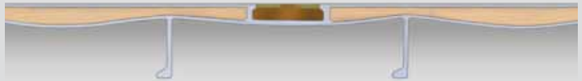
Illustrative cross section showing new top plate and elastomer core of SPS Overlay. In spite of diminution and 'dishing', the original deck plate can be retained to form the bottom plate of the sandwich. New lashing pots are integrated during process.
