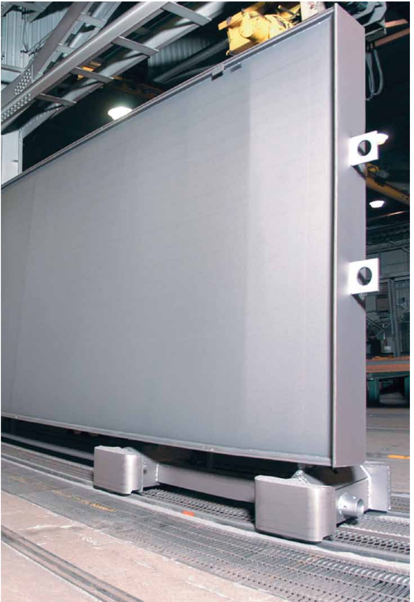
SPS Bridge Deck panel in production
