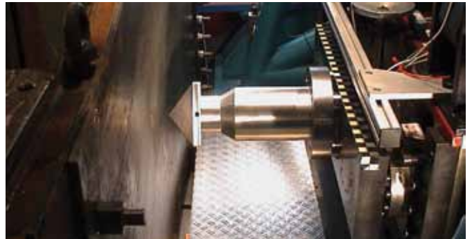
SPS impact test - sharp point-load on a 2 tonne sled striking SPS plate at 5m per second. SPS sustained minor indentation; the all-steel alternative was punctured through.
